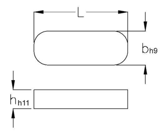
b = 10 h = 8 L = 63.0Tolerance b = 0.036Tolerance h = 0.090
